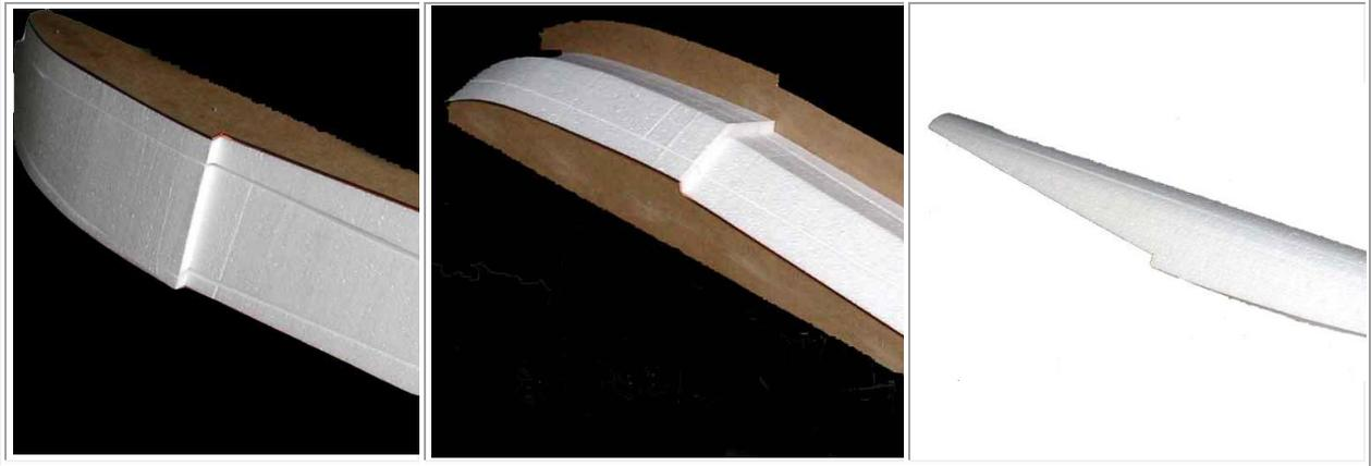
Once the first cut is made, the fat and thin side templates are reversed and a second cut made to get a perfect "Vee". The result is shown above.
