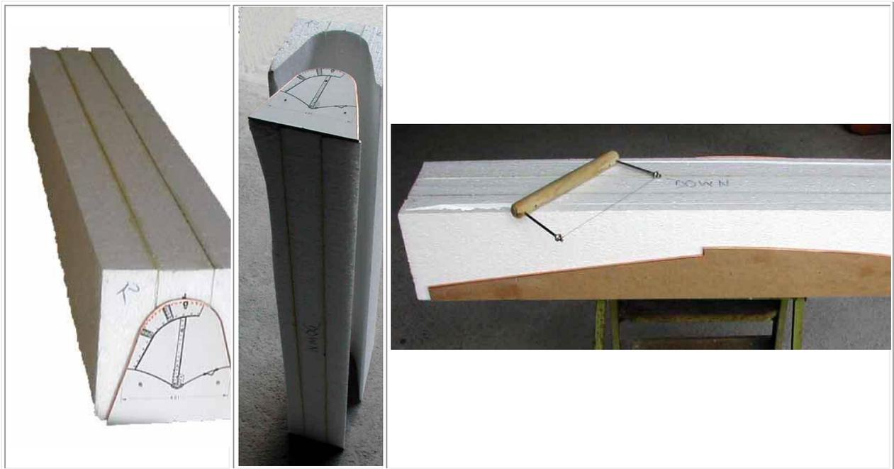
The fundamental difference cutting this style of foam core is the very first step. Templates of the same size and shape are nailed to the back and front of the foam core blank. The hot wire is run around the templates to cut out the equivalent of a "railroad tunnel". The "railroad tunnel" is tacked back onto the hump shape and the fat and thin side templates are tacked onto the outer sides of the "railroad tunnel".
