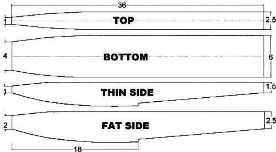
Once you have your templates complete, you will need to drill a series of small holes along the centerline of each template. Into these holes we will insert 2-in. nails that will perforate the foam and hold templates in place while we
